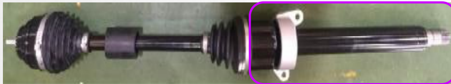
Right Assembly Torsion stiffness: 113\text{Nm}/^\circ
