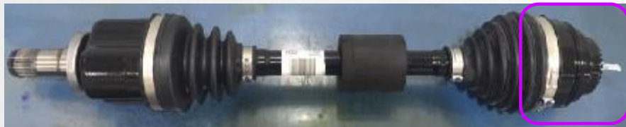
Left Assembly Torsion stiffness: 114\text{Nm}/^\circ
