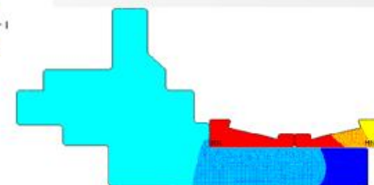
轴承内圈和轮毂过盈配合有限元分析 Finite element analysis of the interference between inner circle of the bearing and the hub
